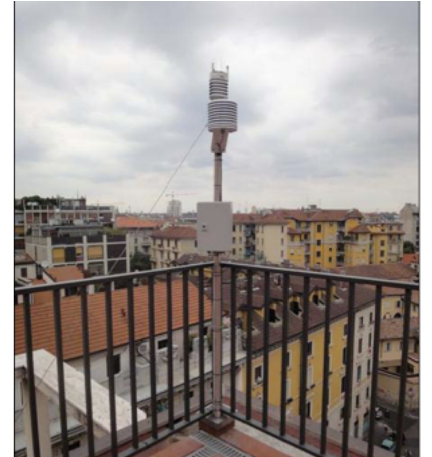
1 = Wind transducers (3 pcs) 2 = Precipitation sensor 3 = Pressure sensor inside the PTU module 4 = Humidity and temperature sensors inside the PTU module
